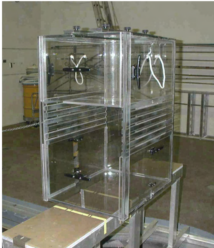
Figure 5. The restrainer used in dosimetric measurements and for irradiation of NHPs in the AFRRRI ^{60}\text{Co} whole-body irradiator. The restrainer's larger sides, identified by white ropes, face a north-south orientation. A PMMA cylinder used to simulate the body of an NHP and to hold the alanine dosimeter package is placed on the first shelf within the restrainer. The restrainer is centered on the table surface. The restrainer is located on a table fitted over a pool of water midway between two carriages containing the ^{60}\text{Co} source rods. The ^{60}\text{Co} rods are stored in cassettes at the bottom of the 15-foot-deep pool when not used.
